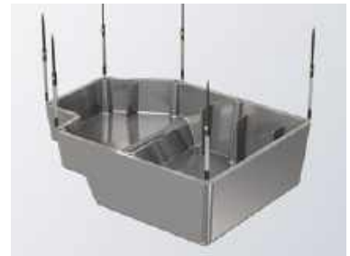
Oil pan flatness measurement
