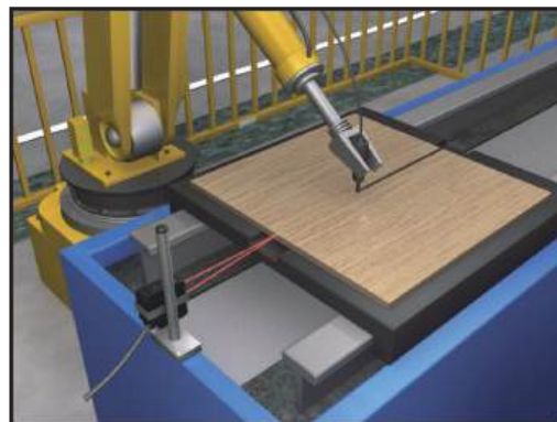
Workpiece detection for woodworking machines
