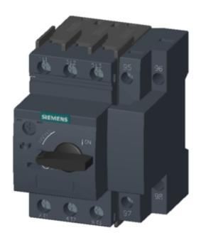
CIRCUIT-BREAKER SZ S00, FOR MOTOR PROTECTION, CLASS 10, W. OVERLOAD RELAY FUNCTION A-RELEASE 7...10A, N-RELEASE130A, SCREW CONNECTION, STANDARD SW. CAPACITY
