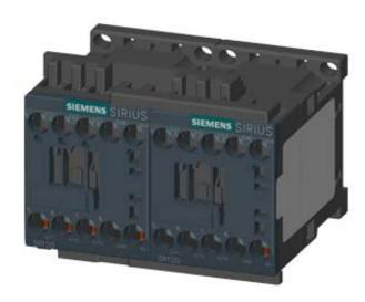
REV. COMB. FOR 3RA27, AC3, 3KW/400V, DC24V 3-POLE, SZ S00 SCREW TERMINAL ELECTR. AND MECH. INTERLOCK
