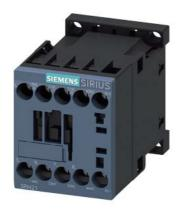
Coupling contactor relay, 2 NO + 2 NC, 24 V DC, 0.7 ... 1.25\* US, Size S00, screw terminal suitable for PLC outputs
