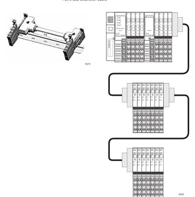
The POINT I/O POINTBus Extension Cable is available in 1 meter and 3 meter lengths as:
