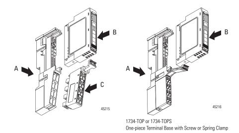
The base (A) mounts onto the DIN rail and provides the backplane. The POINT I/O module (B) snaps into the base. The removable terminal block (C) also snaps into the base and provides the wiring and terminations for field-side connections, as well as system power for the backplane.
