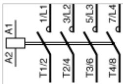
3-Pole Contactors: 3P + N/C
