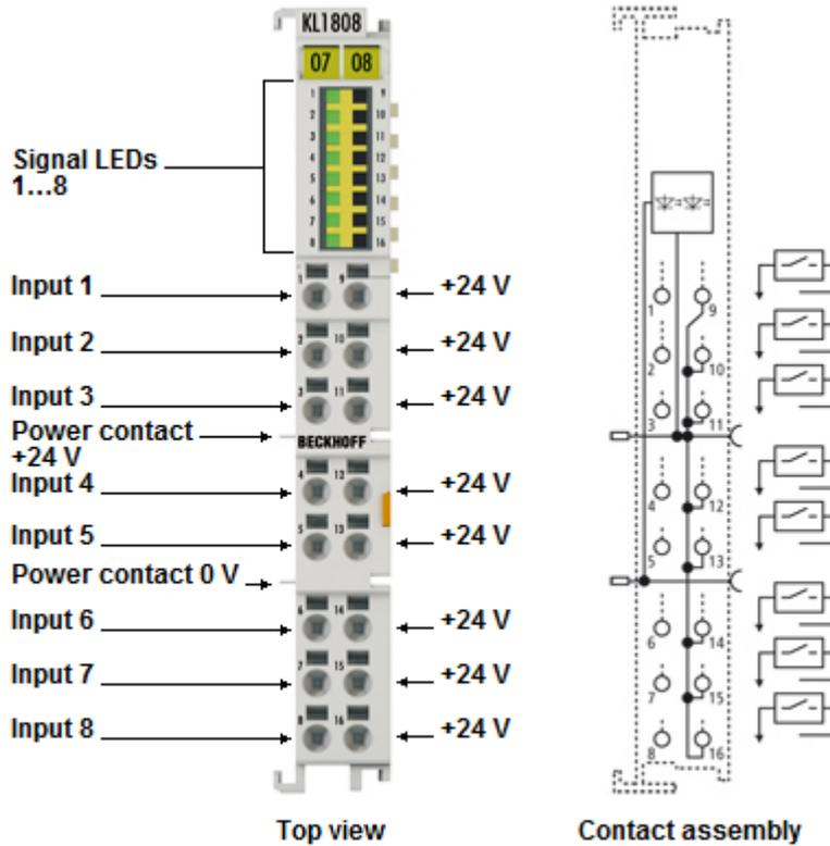
**KL1808 | HD Bus Terminal, 8-channel digital input 24 V DC, 2-wire connection**
