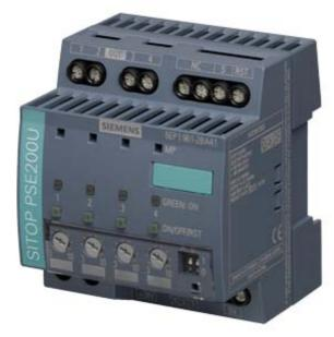
SITOP PSE200U SELECTIVITY MODULE 10A SITOP PSE200U 10 A Selectivity module 4-channel input: 24 V DC/40 A output: 24 V DC/4x 10 A Level adjustable 3-10 A mit status message for each output
