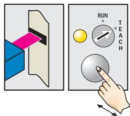
Turn rotary switch to "Teach" position. Press and hold teach-in button > 1 s. Red emitted light and yellow LED flash.
