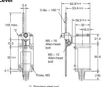
\*1. Stainless steel rod \*2. The head can be mounted in any of the four directions.
