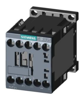
CONTACTOR, AC-3, 3KW/400V, 1NO, AC 230V, 50/60 HZ, 3-POLE, SZ S00 SCREW TERMINAL
