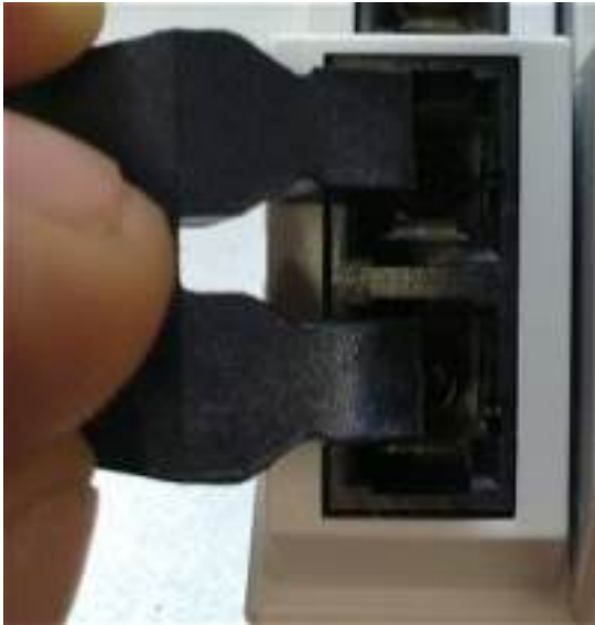
Figure: Blind plugs in unused sockets
