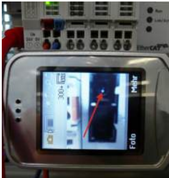
Figure: Visualization of infrared light at the SC duplex connector
