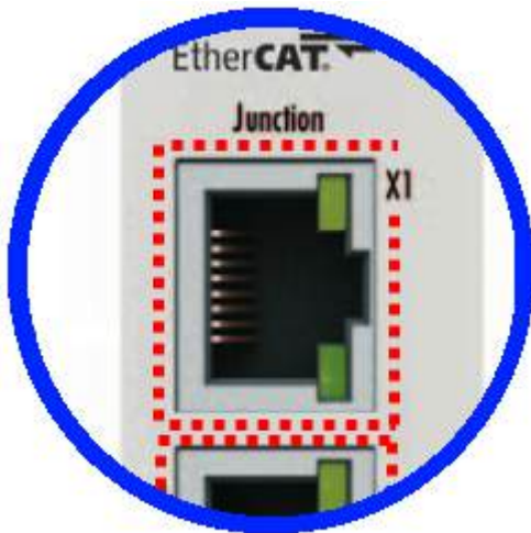
Fig. 11: Identification of FHC port at EK1122-0080 and EK1101-0080
