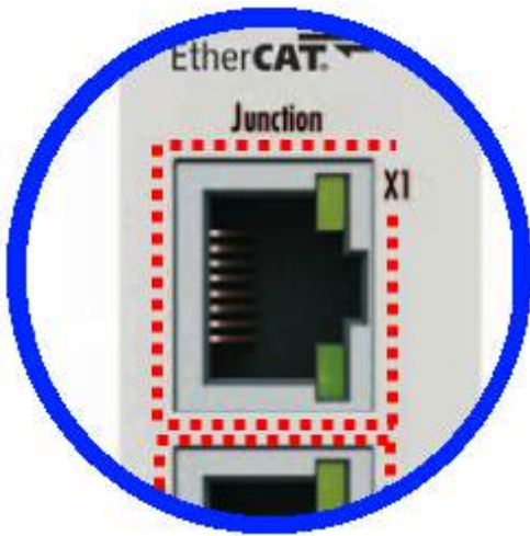
Fig. 10: Fast-Hot-Connect ports at the EK1122-0080
