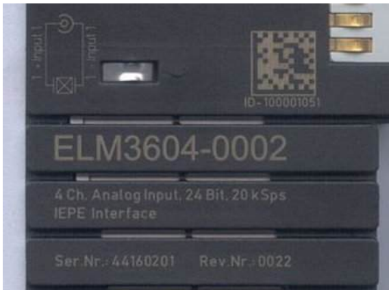
Fig. 8: ELM3604-0002 terminal with unique ID number (QR code) 100001051 and serial/ batch number 44160201
