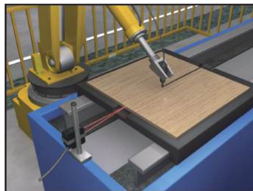
Workpiece detection for woodworking machines
