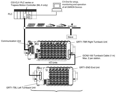
Up to 64 I/O Units can be connected to a Communication Unit.
