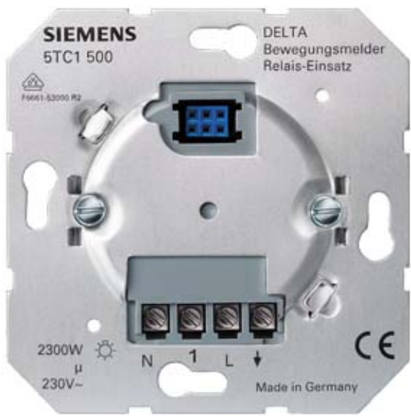
I-SYSTEM MOTION DET. RELAY INSERT 230V 50/60HZ MAX. 2300W 3-WIRE CONNECTION SYSTEM
