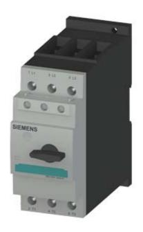
CIRCUIT-BREAKER 28...40 A, N-RELEASE 480 A, SIZE S2, MOTOR PROTECTION CLASS 10 SCREW CONNECTION
