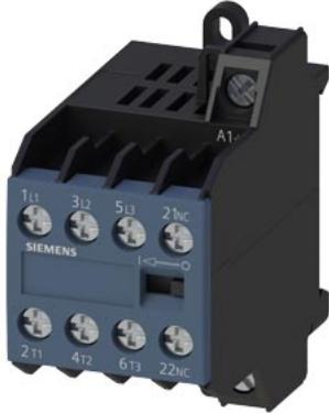
Power relay, AC-3 8.4 A, 4 kW / 400 V 3 NO+1 NC, 24 V DC 3 pole, screw terminal
