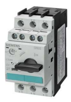
CIRCUIT-BREAKER, SIZE S0, FOR MOTOR PROTECTION, CLASS 10, A REL.1.1...1.6A, N REL.21 A, SCREW CONNECTION, STANDARD BREAKING CAPACITY W. TRANSV. AUX. SWITCH 1NO/1NC
