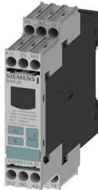
Digital monitoring relay Speed monitoring from 0.1 to 2200 rpm Overshoot and undershoot 24 to 240 V AC/DC 50 to 60 Hz DC and AC ON delay 1 to 900 s Tripping delay 0.1 to 99.9 s Hysteresis 0.1 to 99 rpm 1 change-over contact with or without fault buffer screw terminal Successor product for 3UG3051
