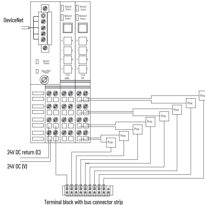
**Figure 6 - Wiring Example of 1734-IV8, 1734-IV8K Using 3-Wire Proximity Switches**
