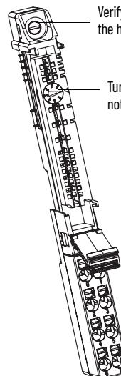
Verify that the DIN rail locking screw is in the horizontal position.
