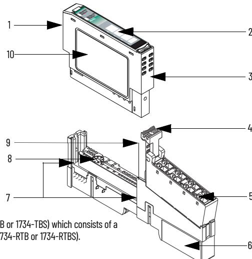
The wiring base assembly includes terminal base, (1734-TB or 1734-TBS) which consists of a mounting base (1734-MB) and removable terminal block (1734-RTB or 1734-RTBS).
