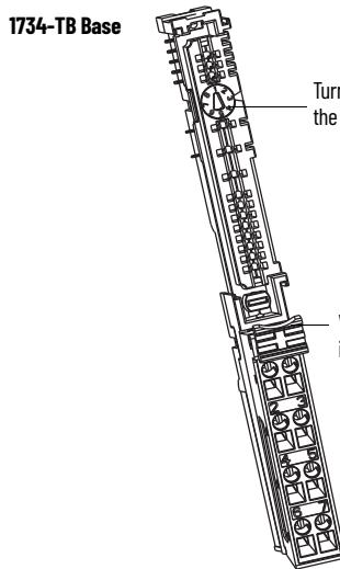
Turn the keyswitch to align the number with the notch. Notch position 3 is shown.
