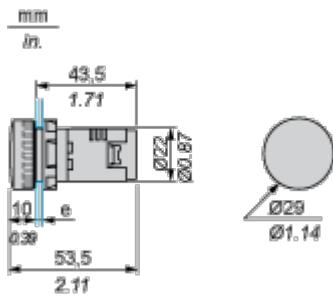
e Support panel thickness: 1 to 6 mm/0.4 to 0.24 in. (metal), 2 to 6 mm/0.8 to 0.24 in. (plastic).
