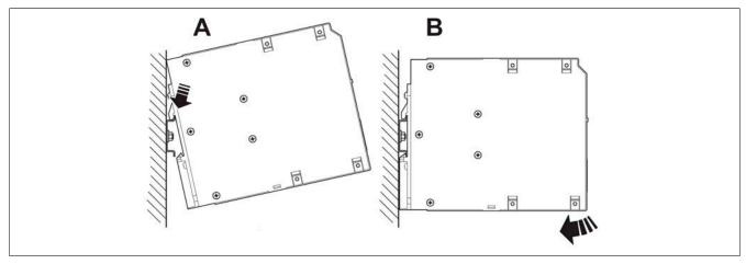
Position the module with the DIN rail guide on the **upper edge** of the DIN rail, and snap it in with a **downward** motion.
