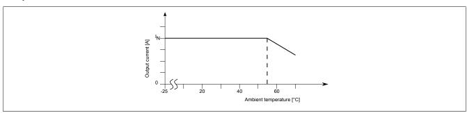
At an ambient temperature of  $55^{\circ}$ C, the unit provides a continuous output current of  $I_{N}$ . At ambient temperatures over  $55^{\circ}$ C, the output power must be derated by 2.5% per Kelvin.
