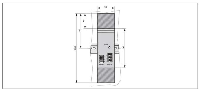
Installation depth 152.5 mm + DIN rail
