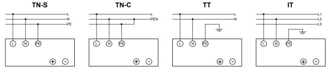
The 100 to 240 VAC connection is made using the L, N and PE screw connections.
