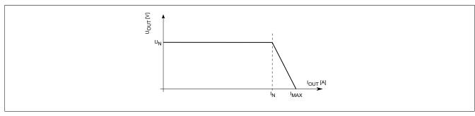
The unit operates according to the U/I characteristic curve. The operating point follows this curve when a load is applied. The output current is limited if a short circuit or overload occurs. Instead of switching off, the unit continues to provide a continuous output current.
