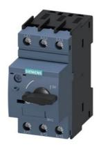
Circuit breaker size S0 for motor protection, CLASS 10 A-release 0.55...0.8 A N-release 10 A screw terminal Standard switching capacity
