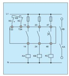
\* Reset button wired in series to feedback loop.
