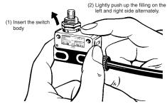
Be sure that the clamp is inserted to the full depth, because the Switch will not function properly if one of the clamps is improperly inserted.
