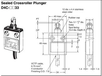
Note: Unless otherwise specified, a tolerance of  $\pm 0.4 \ \text{mm}$  applies to all dimensions.
