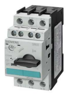
CIRCUIT-BREAKER, SIZE S0, FOR MOTOR PROTECTION, CLASS 10, A REL.0.45...0.63A, N REL.8.2A SCREW CONNECTION, STANDARD BREAKING CAPACITY W. TRANSV. AUX. SWITCH 1NO/1NC
