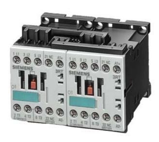
REVERSING CONTACTOR ASSEMBLY AC-3, 4KW/400V, 3-POLE, SZ. S00 SCREW CONNECTION, AC 110V, 50/60 HZ, ELECTR. AND MECH. INTERLOCKING
