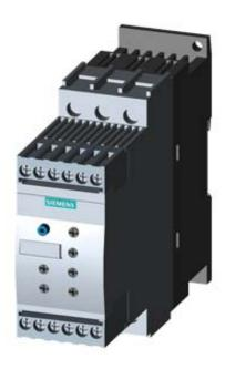
SIRIUS SOFT STARTER, S0, 12.5A, 5.5KW/400V, 40 DEGR., AC 200-480V, AC/DC 24V, SCREW TERMINALS, THERMISTOR MOTOR PROTECTION
