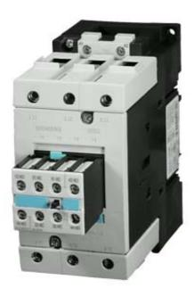
CONTACTOR, AC-3 30 KW/400 V, AC 220V 50/60HZ 2 NO + 2 NC 3-POLE, SIZE S3, SCREW CONNECTION
