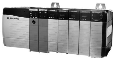
A GuardLogix® controller is a ControlLogix controller that also provides safety control. The GuardLogix system is a dual controller solution—you must use a 1756-L6S/1756-L7S primary controller and a 1756-LSP/1756-L7SP safety partner to achieve up to SIL CL 3/PLe/Cat. 4. A major benefit of this system is that it's still a single project, safety and standard together. The safety partner controller is a part of the system, is automatically configured, and requires no user setup.
