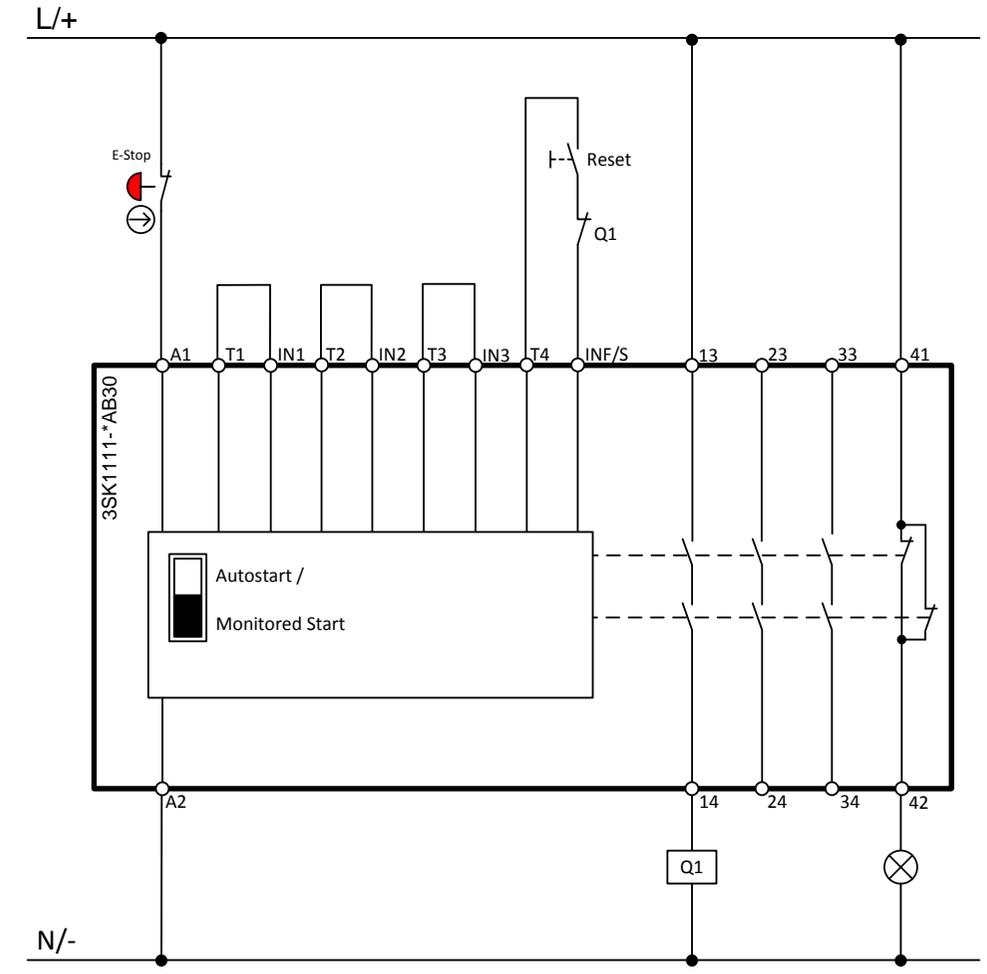
**Wiring diagram 3SK1 Advanced**
