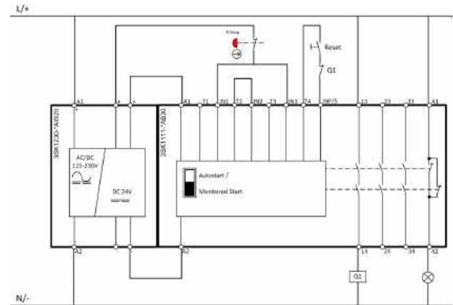
**Wiring diagram 3SK1 Advanced**
