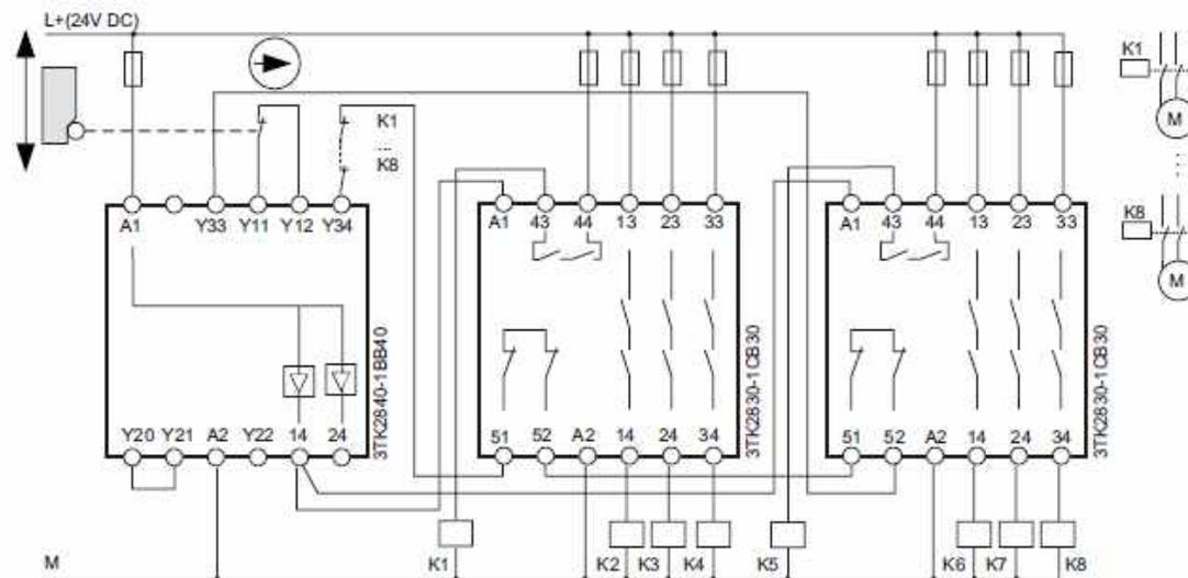
**Wiring diagram 3SK1 Advanced**
