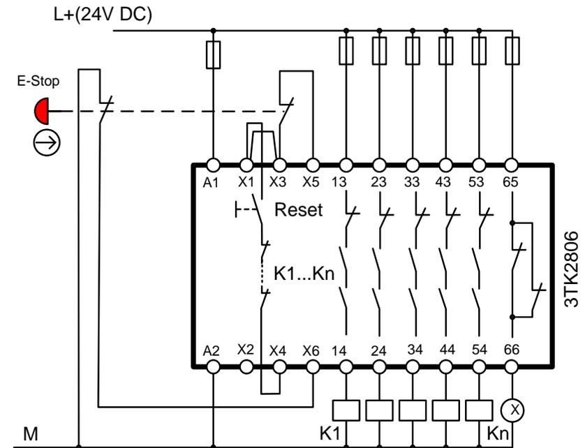
**Wiring diagram 3SK1 Standard**
