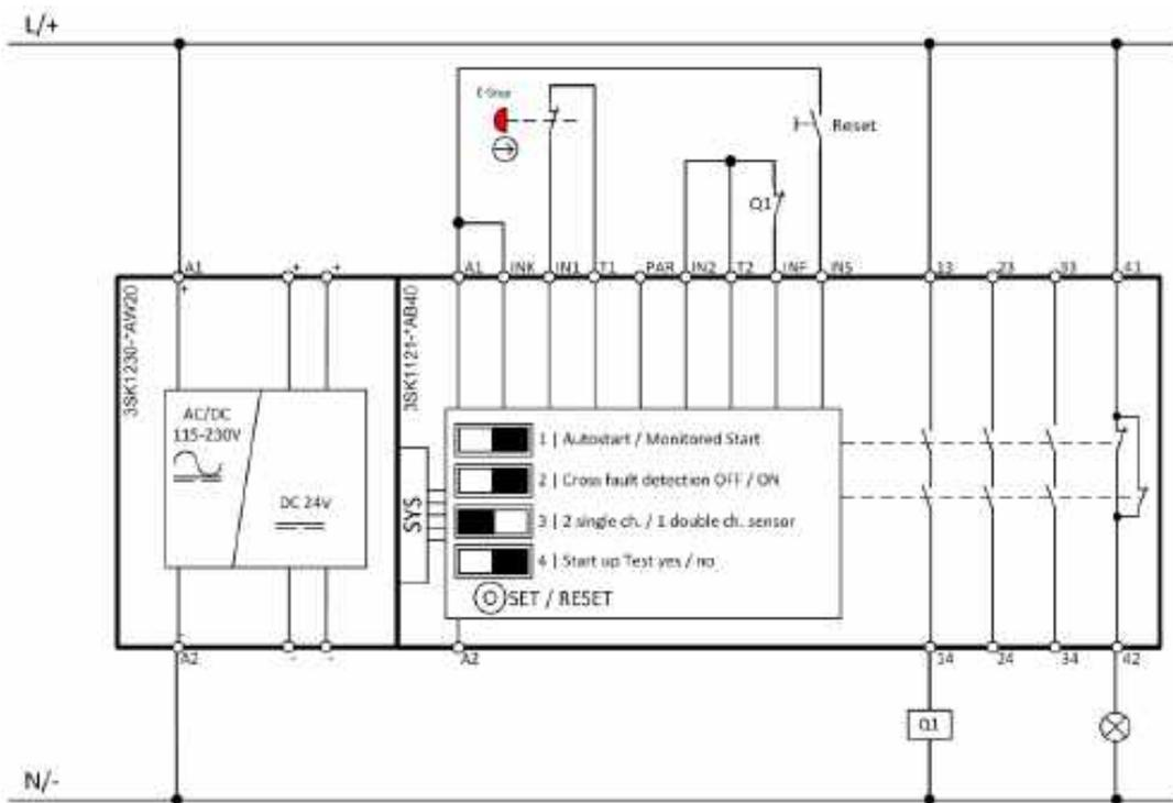
**Example – Usage of 3SK1230 power supply via output terminals +/-**
