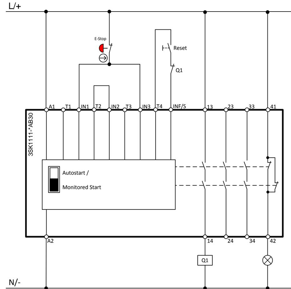
**Wiring diagram 3SK1 Advanced**
