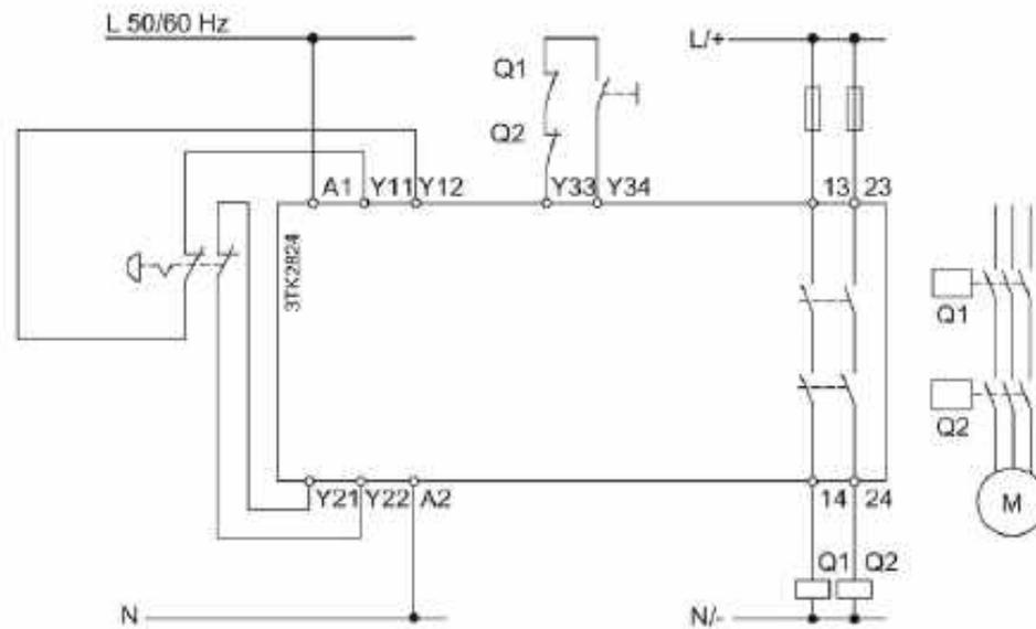
**Wiring diagram 3SK1 Standard**
