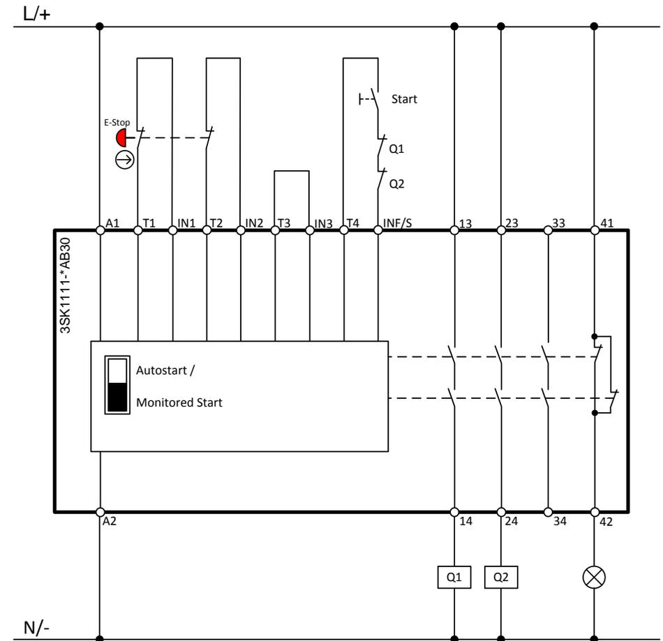
**Wiring diagram 3SK1 Advanced**
