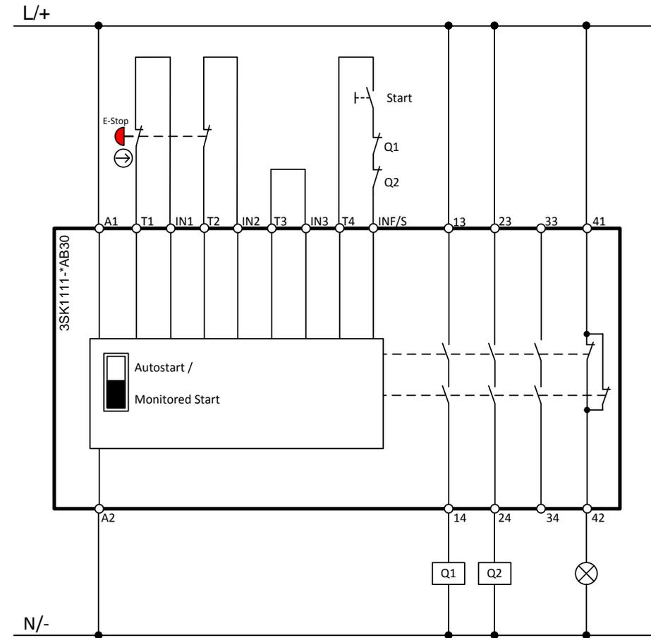
**Wiring diagram 3SK1 Advanced**
