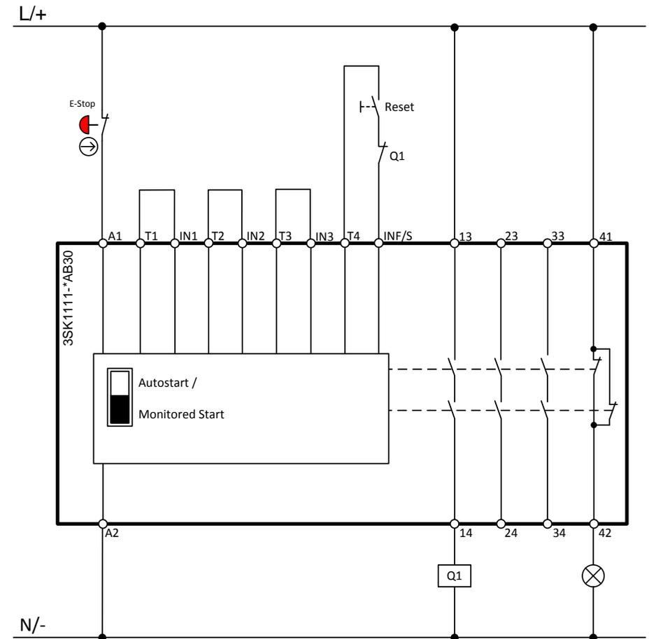
**Wiring diagram 3SK1 Advanced**
