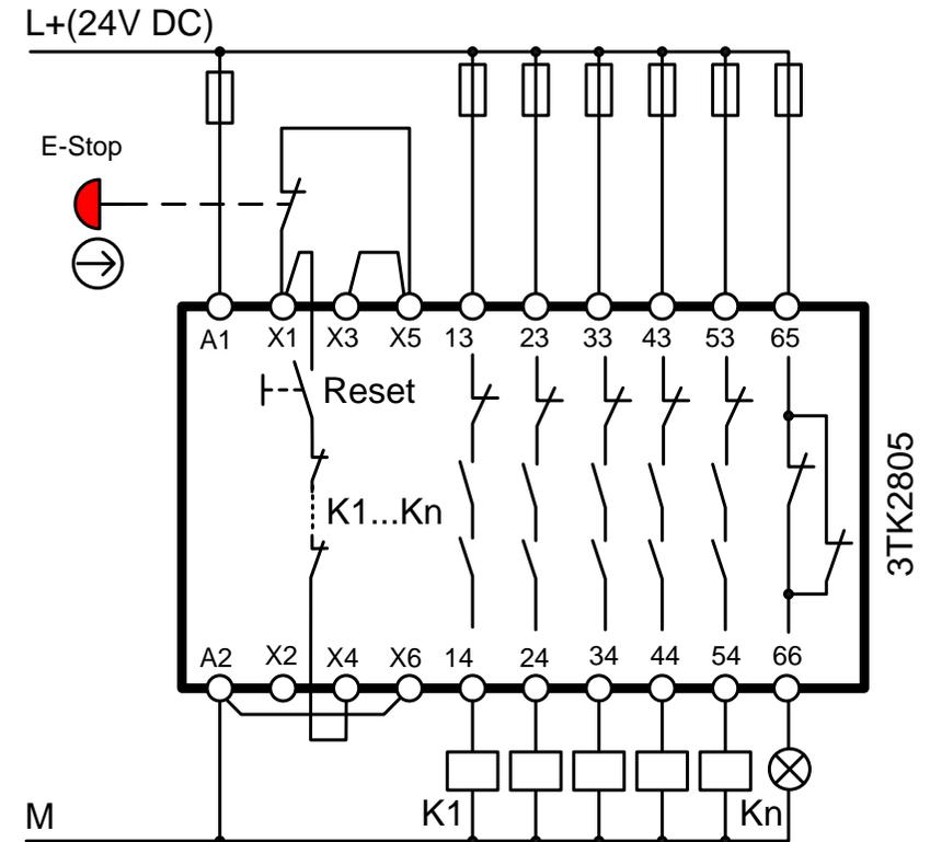
**Wiring diagram 3SK1 Standard**
