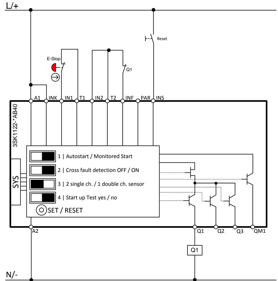
**Wiring diagram 3SK1 Advanced**
