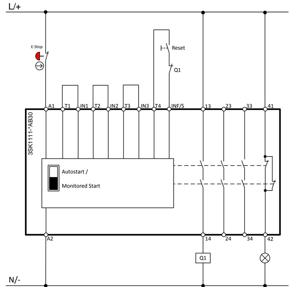
**Wiring diagram 3SK1 Advanced**
