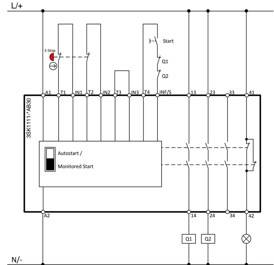
**Wiring diagram 3SK1 Advanced**
