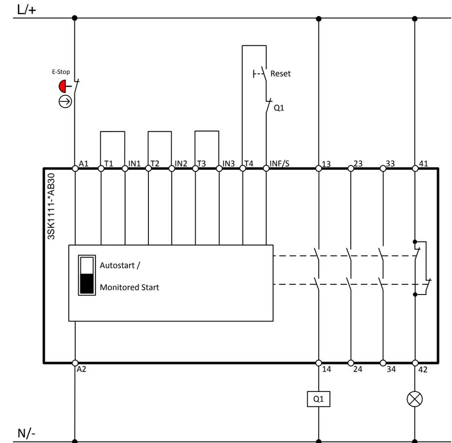
**Wiring diagram 3SK1 Advanced**
