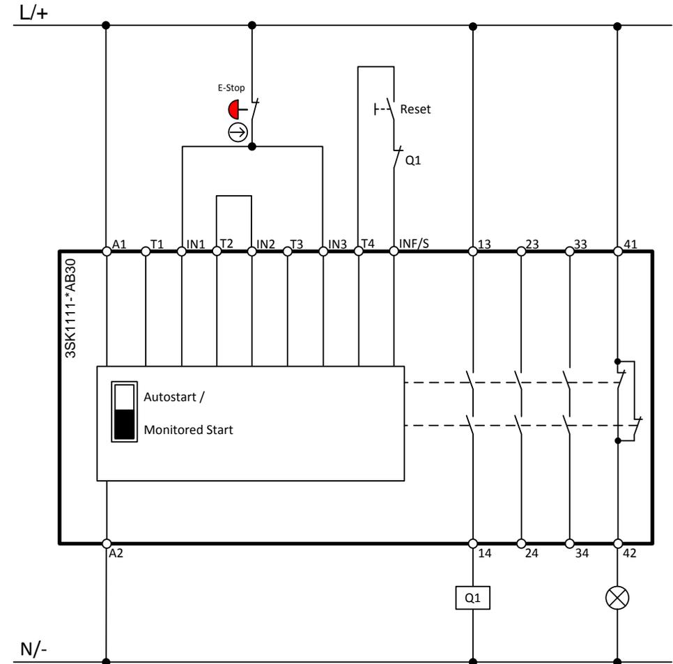
**Wiring diagram 3SK1 Advanced**
