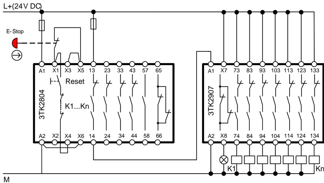
**Wiring diagram 3SK1 Standard**
