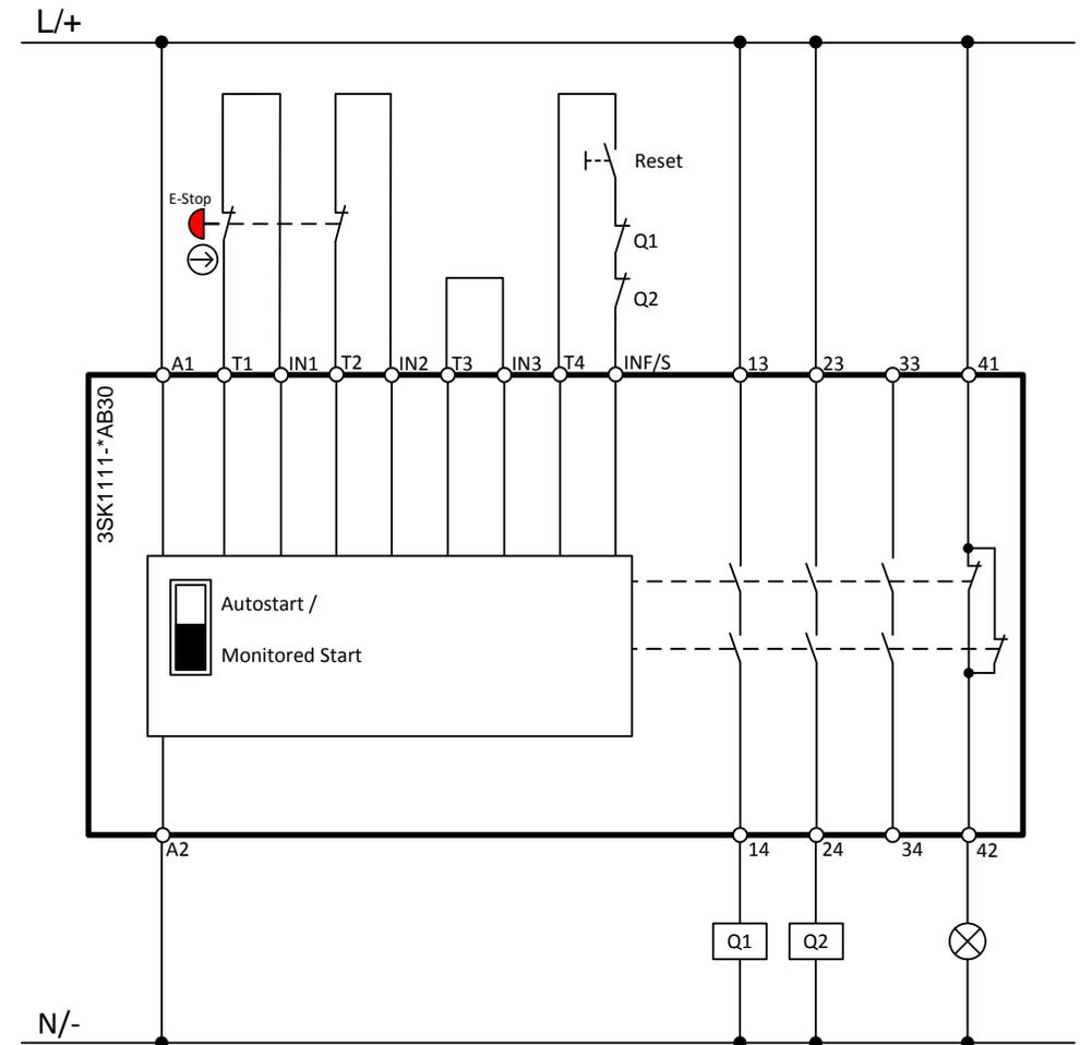
**Wiring diagram 3SK1 Advanced**
