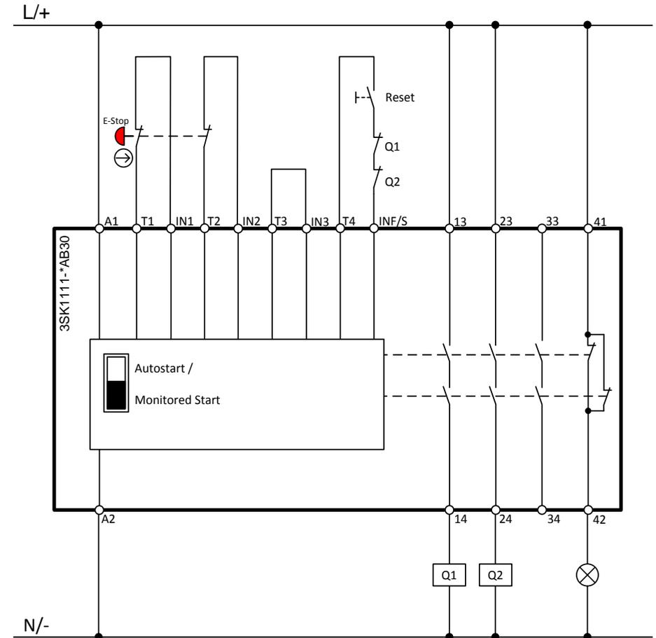
**Wiring diagram 3SK1 Advanced**
