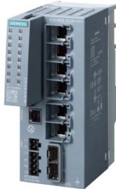
SCALANCE XC206-2SFP manageable Layer 2 IE switch; IEC 62443-4-2 certified; 6x 10/100 Mbit/s RJ45 ports; 2x 100/1000 Mbit/s SFP; 1x console port; diagnostics LED; redundant power supply; temperature range -40 °C to +70 °C; assembly: DIN rail/S7 mounting rail/wall Office redundancy functions features (RSTP, VLAN,...); PROFINET IO device; Ethernet/IP-compliant; C-plug slot;
