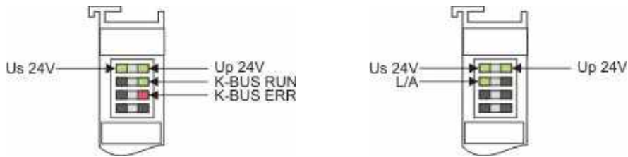
Operation with K-bus terminals
