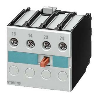
AUXILIARY SWITCH BLOCK, 2 NO, DIN EN 50005, CABLE ENTRY FROM ABOVE SCREW CONNECTION, FOR CONTACTORS FOR SWITCHING MOTORS, 2-POLE
