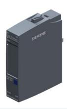
SIMATIC ET 200SP, Analog input module, Al 2x U/l 2-.4-wire High Feat., suitable for BU type A0, A1, Color code CC05, channel diagnostics, 16 bit,  $\pm$ 0.1%
