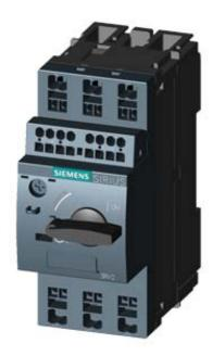
CIRCUIT-BREAKER SZ S00, FOR MOTOR PROTECTION, CLASS 10, A-RELEASE 4.5...6.3A, N-RELEASE 82A SPRING-L. CONNECTION, STANDARD SW. CAPACITY W. TRANSVERSE AUX. SWITCH 1NO+1NC
