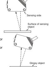
If the sensing object has a glossy surface, however, incline the Sensor by 5° to 10° as shown in the illustration, provided that the Sensor is not influenced by background objects.
