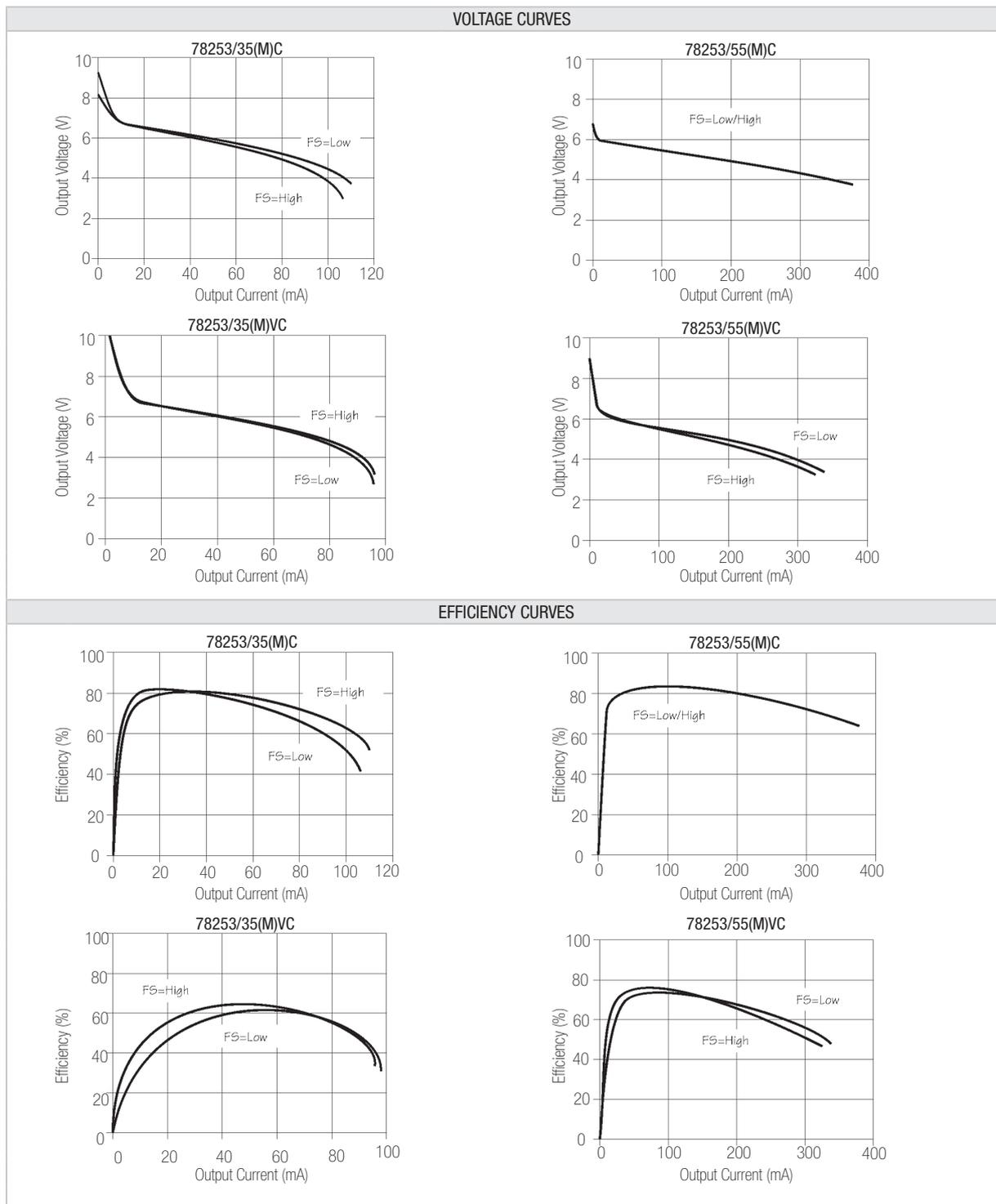
All curves are derived from testing with the Maxim MAX235 IC using the circuit shown in application note MPAN-03 (download at <http://www.murata-ps.com/data/apnotes/mpan-03.pdf>).
