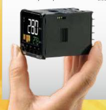
Thanks to the IP66 protection\*3 of the front cover, the E5\_C can withstand humid environments and also be cleaned with non-aggressive fluids.
