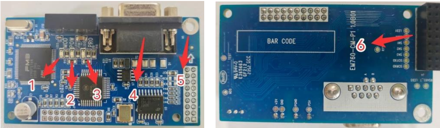
Figure 2.1.1 Front view Figure 2.1.2 Back view 1. MODBUS indicator 2. POWER indicator 3. PROFIBUS indicator 4. PROFIBUS DP interface 5. Screw positioning hole 6. Inverter interface
