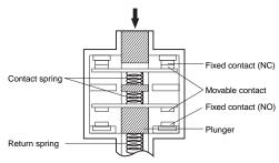
Conforms to EN60947-5-1 Direct Opening Operation ⊕
