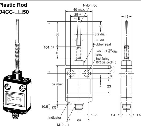
\*1. Operation is possible in any direction except parallel to the axis ↓.
