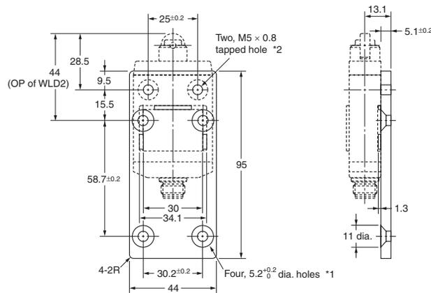
Note: Four hexagonal flat head bolts (M5 × 0.8, length: 10) and two Allen-head bolts (M5 × 0.8, length: 15) are included.
