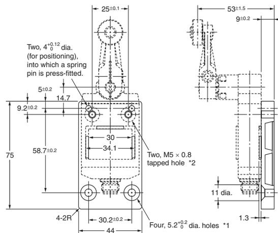
Note: Four hexagonal flat head bolts (M5 × 0.8, length: 10), two Allen-head bolts (M5 × 0.8, length: 15), and two spring pins (4 × 14) are included.
