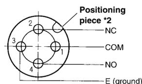
\*1. "Lit when not actuated" means that when the actuator is in the free position, the indicator is lit, and when the actuator is turned or pushed and the contact comes into contact with the NO side, the indicator turns OFF.
