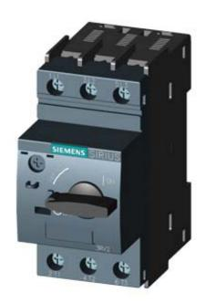
CIRCUIT-BREAKER SZ S0, FOR MOTOR PROTECTION, CLASS 10, A-REL. 0.9...1.25A, N-REL. 16A SCREW CONNECTION, STANDARD SW. CAPACITY
