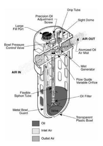
The air flow then carries the oil to the pneumatic devices where the lubricant mist coats the moving and sliding surfaces thus reducing friction and wear.
