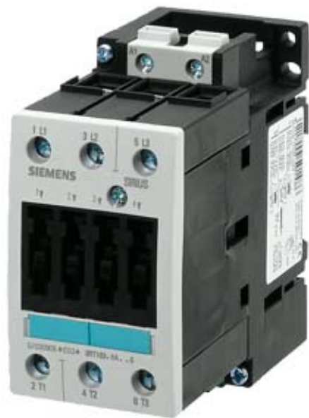
CONTACTOR, AC-3 15 KW/400 V, AC 110V 50/60HZ, 3-POLE, SIZE S2, SCREW CONNECTION
