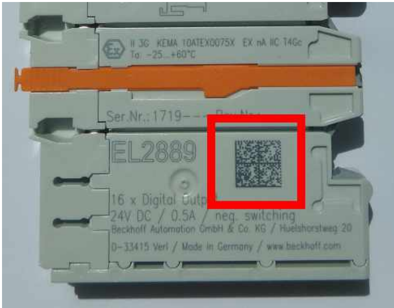
Fig. 29: BIC as data matrix code (DMC, code scheme ECC200)
