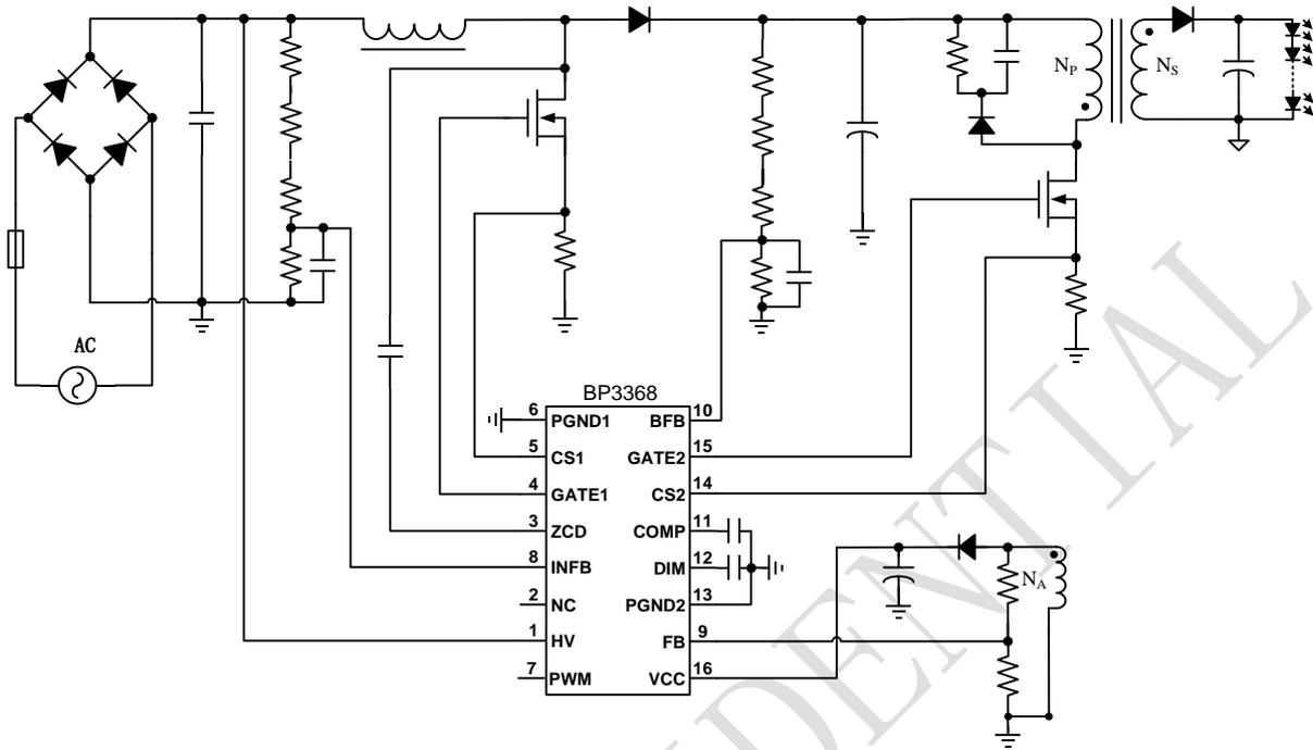
Fig.1 BP3368 for Non-Dimming Application
